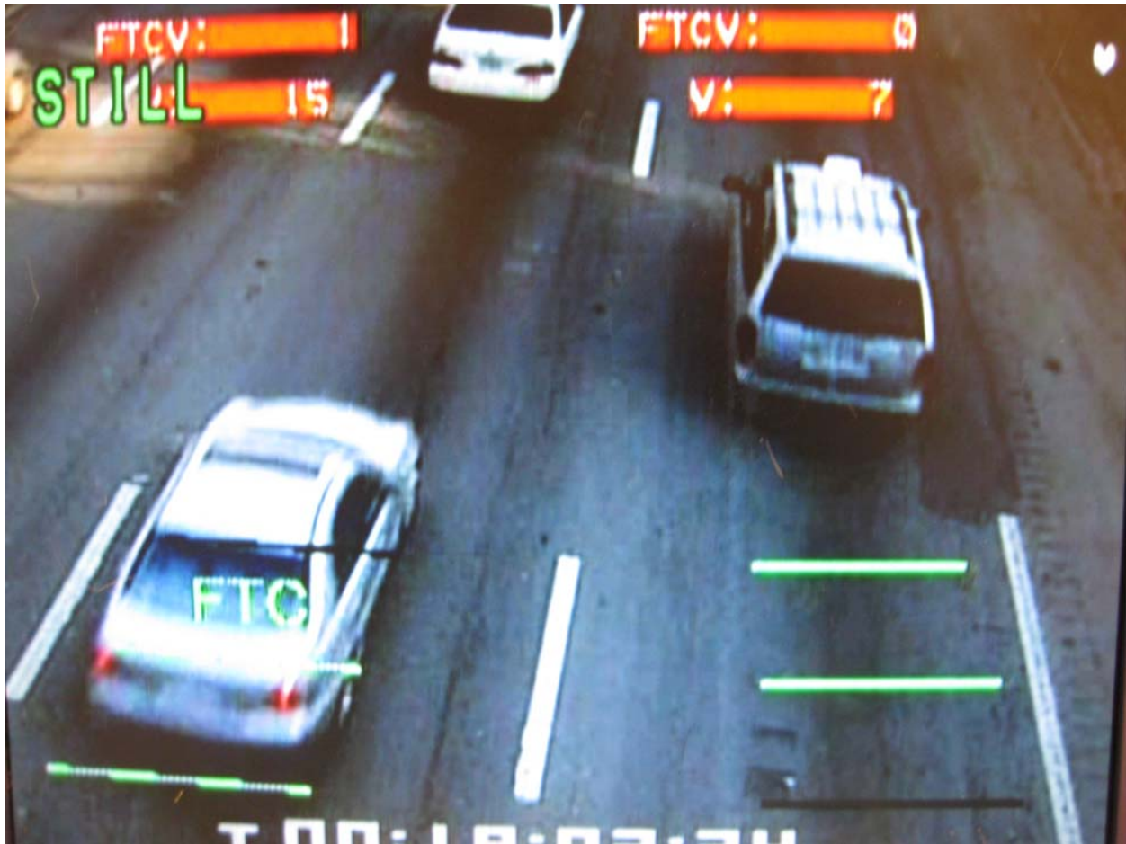
1 2 Figure 3: Screenshot of Autoscope Video Algorithm for one of the Test Sites 3
